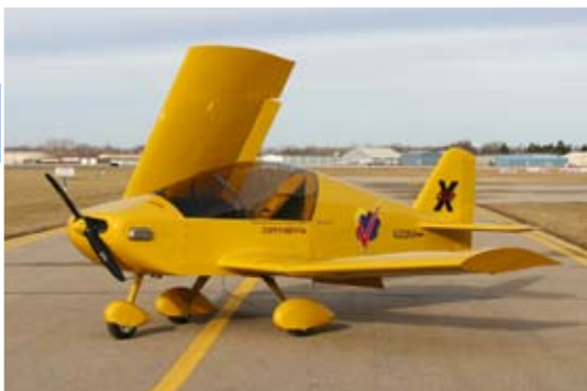
Version tricycle, ailes repliables (Photo Sonex Aircraft)
