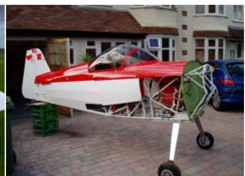
Fuselage en tubes (Photo Todds)
