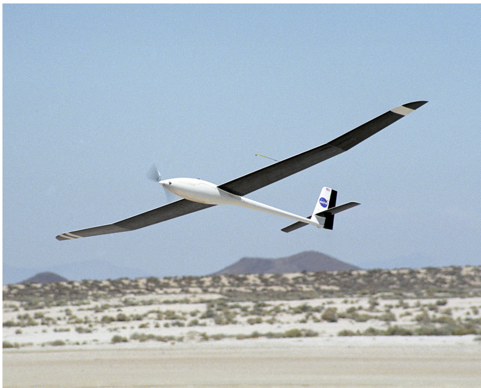
Figure 1. The Cloud Swift UAV. The Cloud Swift is a modified SBXC glider (RnR Products) and has a span of 4.27 m (14 ft) and a weight of 6.8 kg (15 lb).
